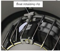
Tighten until snug with a Phillips Head screw driver and repeat for 3 remaining screws.
