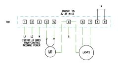
\* REMOVE FACTORY INSTALLED AUX INTERLOCK JUMPER WIRE FROM TB1:8 AND TB1:9 IF EXTERNAL DEVICE IS REQUIRED. THE EXTERNAL INTERLOCK DEVICE (WIND CONTROLLER, LEVEL CONTROLLER, REMOTE SWITCH, ETC.) NON POWERED DRY CONTACT (NORMALLY CLOSED) MUST PROVIDE DELAY CIRCUITRY TO PREVENT AERATOR SHORT CYCLING, FAILURE TO DO SO WILL CAUSE AERATOR DAMAGE.
